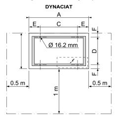
Free space to be maintained to allow sufficient room for maintenance of the unit.
